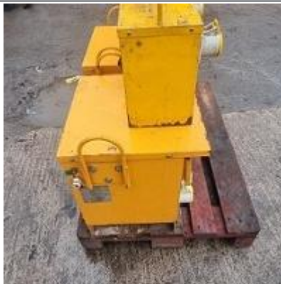
Pallet of 110V Transformers
